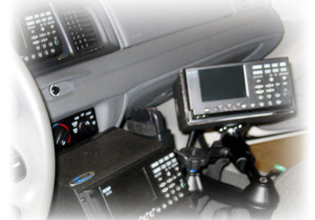
Passenger-Side Arm Mount (used when MDTs or laptops inhibit in-dash mounting)
